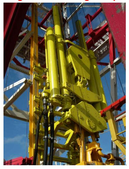
Control Flow's newest Drill String Compensator features the latest and most improved technology in the industry. The benefits are lighter weight, improved operational reliability, and better "Weight On Bit "performance. Available in both 20 and 25 foot stroke lengths, this new DSC is suitable for both new installations and upgrades of your present Drilling Package.
